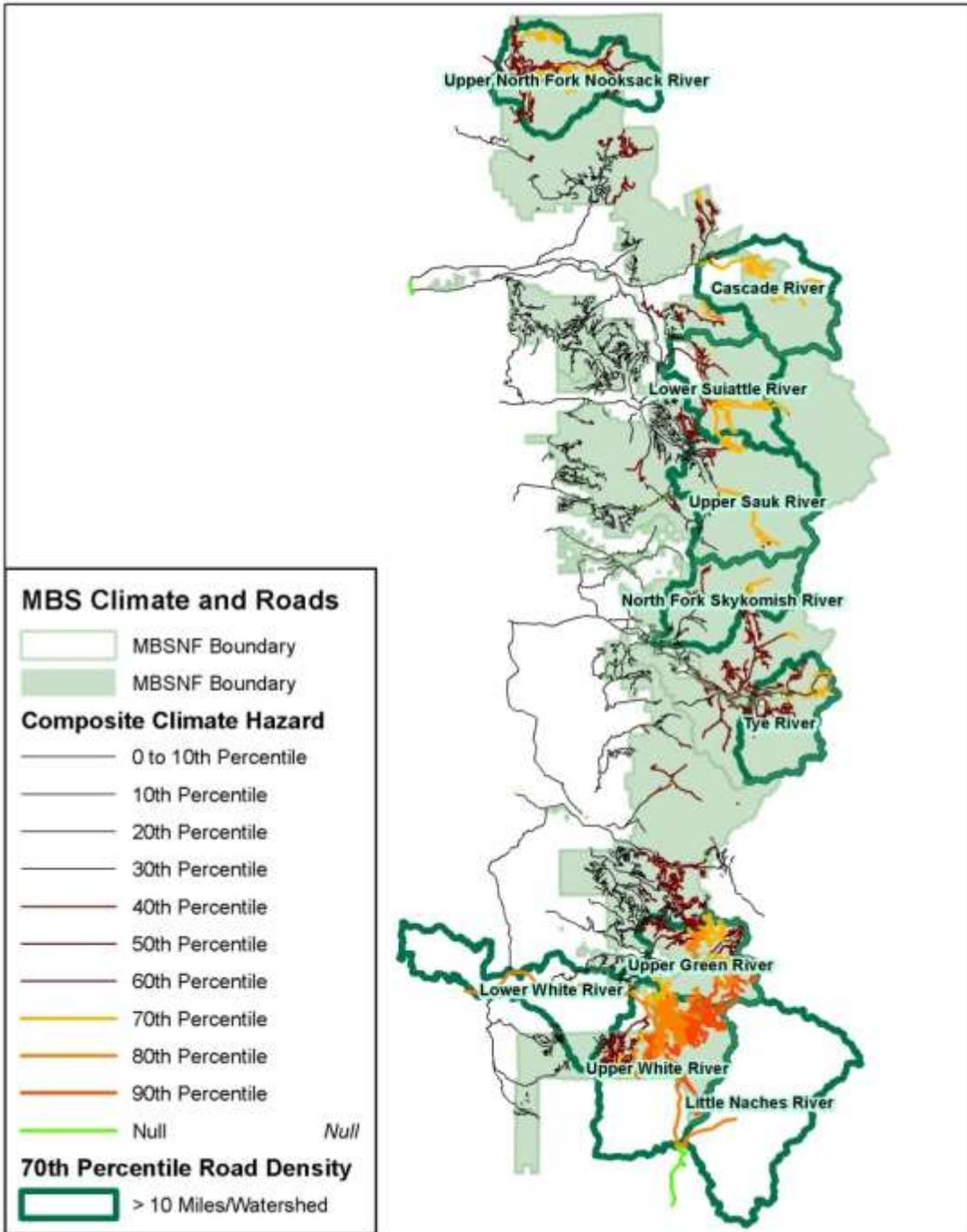
Figure 5. Composite climate hazard scores for road segments on the MBSNF. Watersheds with more than 10 miles of road exceeding the 70<sup>th</sup> percentile scores are outlined in dark green.
