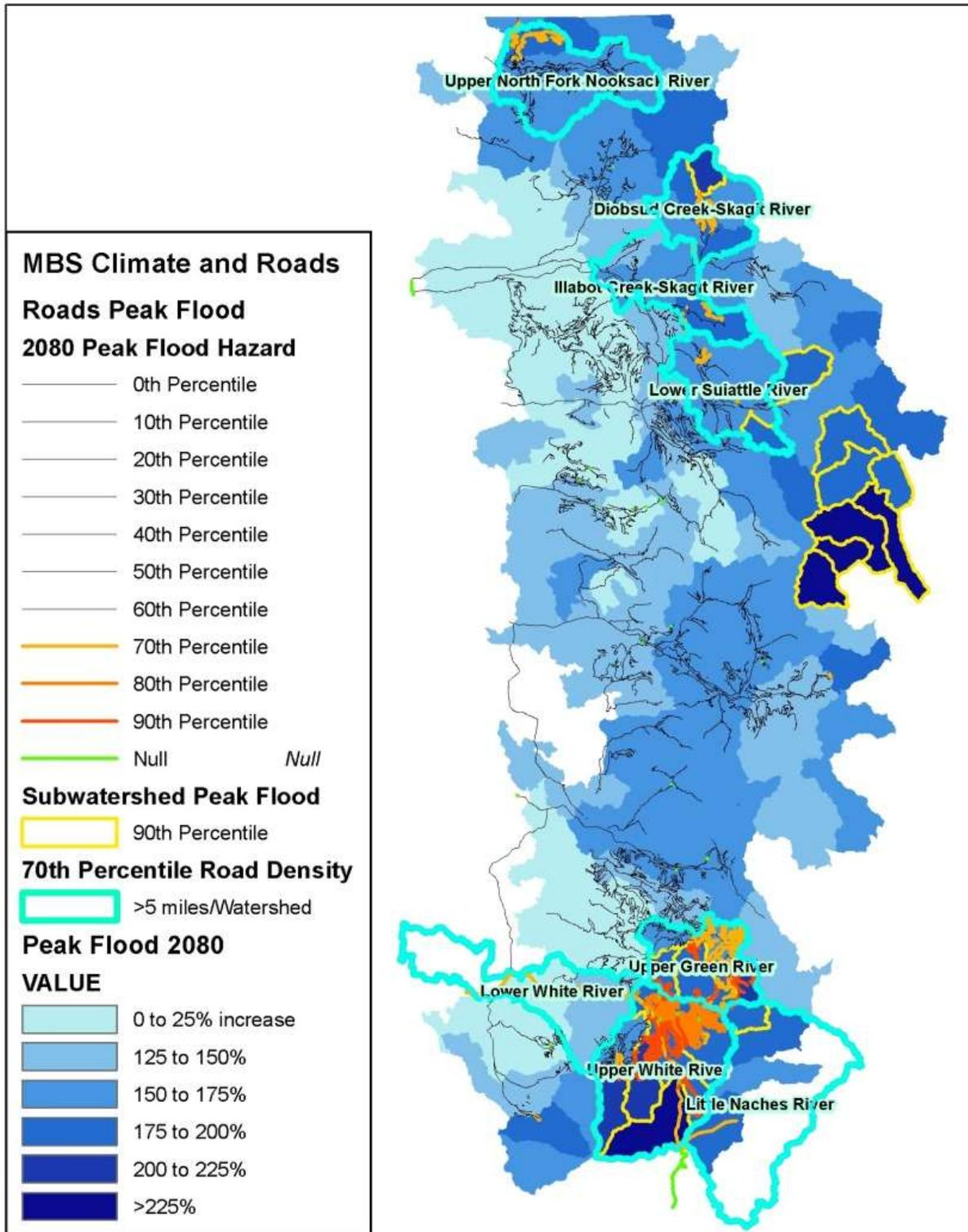
Figure 1. Potential 2080 peak flood level scores overlaid onto watershed and subwatershed boundaries. Watersheds with more than 5 miles of roads exceeding the 70<sup>th</sup> percentile are highlighted in blue. Subwatersheds with peak 2080 flood levels above the 90<sup>th</sup> percentile are outlined in yellow.
