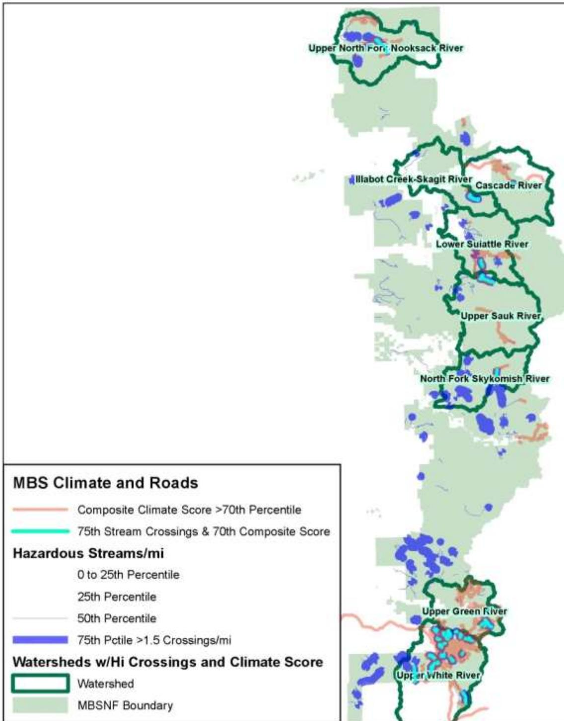
Figure 9. Roads ranked by the 75<sup>th</sup> percentile of the density of hazardous stream crossings per mile (thick blue lines), overlaid by the 70<sup>th</sup> percentile composite road hazard scores (thick red line). Bright blue lines outlined in purple indicate roads that have both high density of hazardous crossings and high hazard scores. Watersheds that contain these overlapping roads are outlined in dark green.
